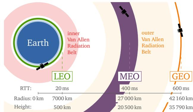
**Figure 2.1** – The Most Important Earth Orbits: Geostationary Earth Orbit (GEO), Low Earth Orbit (LEO), Medium Earth Orbit (MEO), and the inner and outer Van Allen radiation belts, zones of energetic charged particles, which makes it impracticable for satellites.
