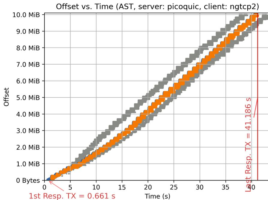
**Figure 5.17** – Trace of *Picoquic* and *Ngtcp2* in ASTRA Scenario with a Conspicuous Number of Retransmissions
